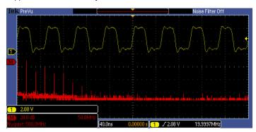
Figure 4: Analyze - FFT analysis of a pulsed signal. A comprehensive set of integrated analysis tools speeds verification of your design's performance.
