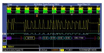
Figure 7: Search step 2: Wave Inspector automatically searches through the record and marks each event with a hollow white triangle. You can then use the **Previous** and **Next** buttons to jump from one event to the next.
