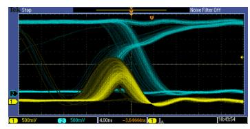
Figure 8: Digital phosphor technology enables a 5,000 wfm/s waveform capture rate and real-time intensity grading on the MSO/DPO2000B Series.
