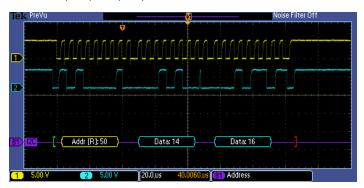
Figure 14: Triggering on a specific data packet going across an  $l^2$  C bus. The yellow waveform is clock and the blue waveform is data. A bus waveform provides decoded packet content including Start, Address, Read/Write, Data, and Stop.
