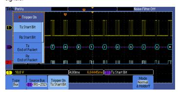
Figure 2: Capture - Triggering on a specific transmit data packet going across an RS-232 bus. A complete set of triggers, including triggers for specific serial packet content, ensures you quickly capture your event of interest.
