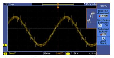
Figure 13: Output of DAC Signal - Notice how FilterVu™ clearly shows the noise-free steps of the DAC in the foreground trace (yellow) which has removed all frequencies above 5.5 kHz. FilterVu also captures and displays high-frequency glitches up to the full bandwidth of the oscilloscope in the background trace (orange).
