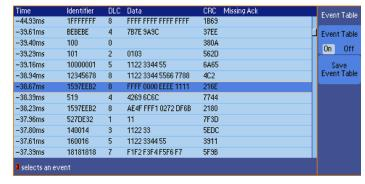
Figure 15: Event table showing decoded Identifier, DLC, DATA, and CRC for every CAN packet in a long acquisition.
