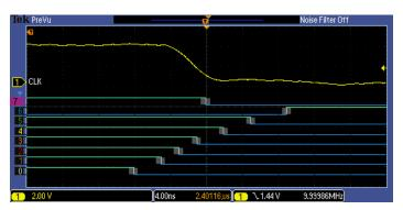
Figure 11: White edges indicate additional information is available by acquiring at a higher sample rate.
