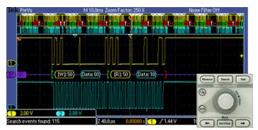
Figure 3: Search - I<sup>2</sup>C decode showing results from a Wave Inspector search for Address value 50. Wave Inspector controls provide unprecedented efficiency in viewing and navigating waveform data.
