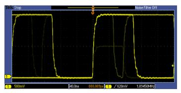
Figure 1: Discover - A waveform capture rate of 5,000 wfm/s maximizes the probability of capturing exclusive glitches and other infrequent events.
