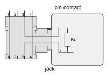
If the 'signal'-line in your transmitter is not assigned to contact 3, please do not forget to adjust the logger-angle-type plug and the external angle-type plug accordingly:
