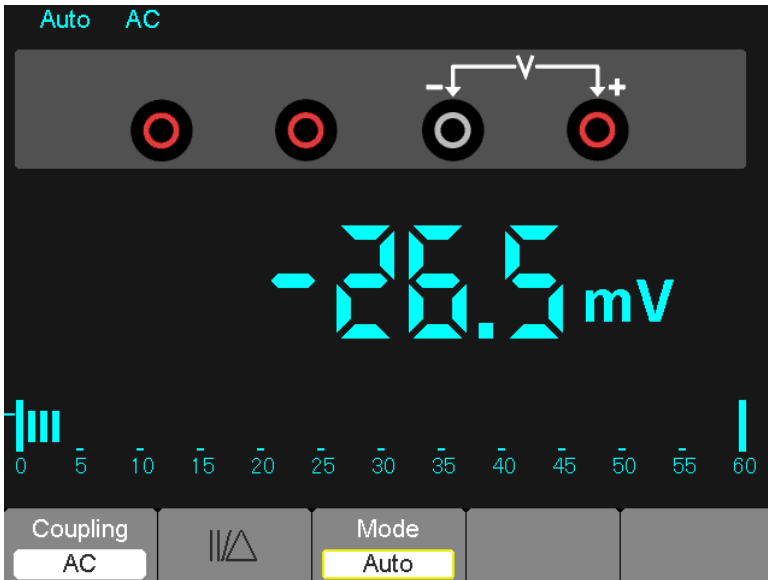
Figure 7-7 AC voltage Measurement
