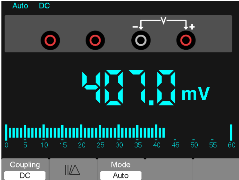
Figure 7-6 DC voltage Measurement
