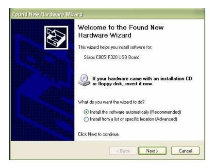
Make sure the program disk is still in the PC CD-ROM drive. Select the 'recommended' installation and follow the on-screen prompts to complete the driver installation. If this is a repeat connection of the RHT50 to the USB port, the driver installation process will be automatically skipped.
