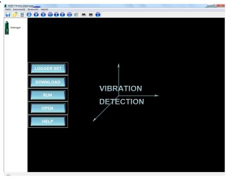
The five large buttons on the left side of the software screen can be used to configure the datalogger (Logger Set), transfer data from the datalogger to the PC (Download), record real-time data (Run), open a file (Open), or view the help utility or software version (Help). These functions are also available on the window's menu items and smaller control icons at the top of the window. These menus and icons are explained in detail below.
