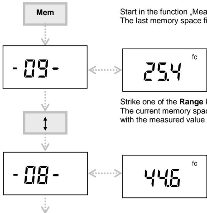
Start in the function „Measuring“ and press down the key **Mem**.
