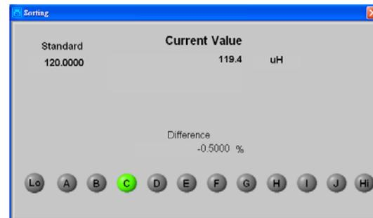
The screenshot shows the 'Sorting' window. It displays 'Standard' as 120.0000 and 'Current Value' as 119.4 uH. Below that, it shows 'Difference' as -0.5000 %. At the bottom, there is a row of buttons labeled 'Lo', 'A', 'B', 'C', 'D', 'E', 'F', 'G', 'H', 'I', 'J', and 'Hi'. The 'C' button is highlighted in green.
