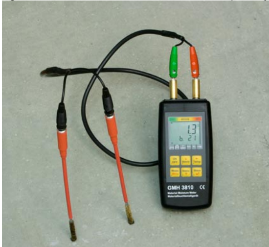
Measuring concrete with brush probe GBSL91
