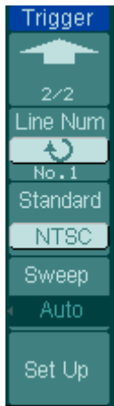
Figure 2- 46 Table 2- 24 The Video Trigger menu (Page 2/2, when Sync is set as the specified line)
