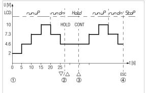
**Interval parameters:** output quantity: U (range of 0 ... 15 V),  $5 \pm Rr \pm 2$  V, End = 10 V, number of interval steps = 3, E = 5 s,  $RadE = Ru \pm a$
