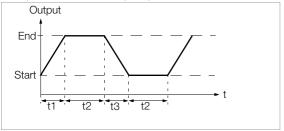
Manually Controlled Ramp Sequence After entering all parameters, start with  $\underbrace{\text{OUT}}_{\text{ENTER}}$ . Rising or falling ramps can be triggered with the  $\triangle$  or  $\nabla$  key.
