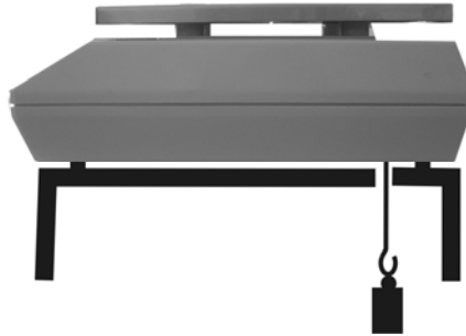
Fig. 1: Setup of balance for underfloor weighing
