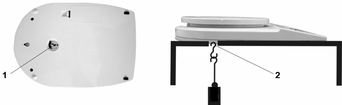
Fig. 1: Setting up the balance for underfloor weighings
