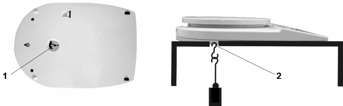
Fig. 1: Setting up the balance for underfloor weighings
