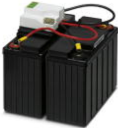
Power storage device, lead AGM, VRLA technology, 24 V DC, 13 Ah, tool-free battery replacement, automatic detection, and communication with QUINT UPS-IQ
