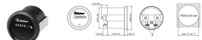
1 Electrical connection: +/~ left, -/~ right (rear view) Front bezel thickness max. 6 [0.24] without having to shorten the clamping bracket
