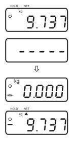
Put the test objects subsequently on the weighing plate, the respective deviation from the nominal weight is displayed with the respective sign to "+" and "-" (e.g. + 0.037 g).
