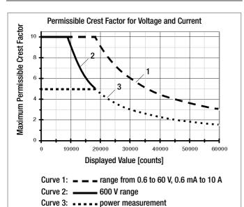
Above figure: Influence of Crest Factor on Display Range Additional error caused by the signal's crest factor:
