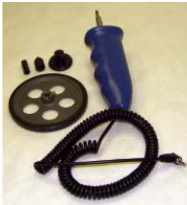
Remote Infrared Sensor (IRS-P) Gap 0.50 inches
