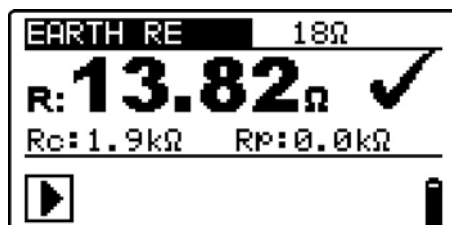
Figure 5.32: Example of earth resistance measurement result
