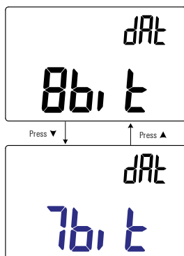
Figure 3-12 Changing the data bits
