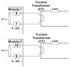
Two EMI-420  $\sim$  CT input modules can not be plugged in Module-1 and Module-2 socket at the same time.
