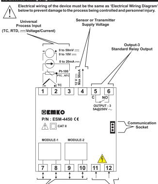
Optional Input/Output Module Terminals Relay, SSR Driver, Digital or Current Output Module
