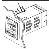
The unit is designed for panel mounting.
