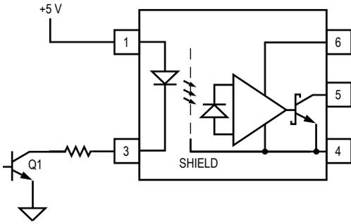
Figure 19. Not Recommended Open Collector LED Drive Circuit.
