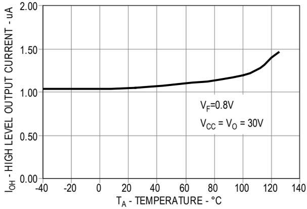
Figure 4. High Level Output Current vs. Temperature.
