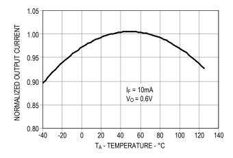
Figure 3. Normalized Output Current vs. Temperature.
