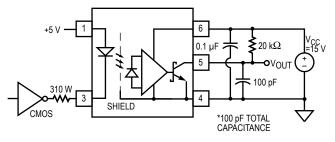
Figure 13. Recommended LED Drive Circuit.
