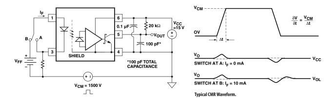
Figure 7. CMR Test Circuit.
