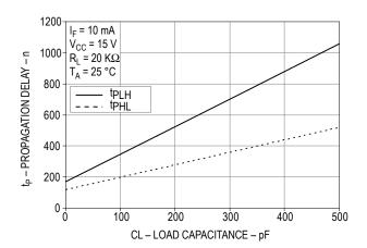
Figure 10. Propagation Delay vs. Load Capacitance.
