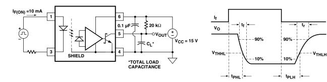
Figure 6. Propagation Delay Test Circuit.
