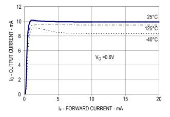
Figure 2. Typical Transfer Characteristics.
