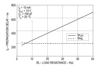
I<sub>F</sub> = 10 mA C<sub>L</sub> = 100 pF R<sub>L</sub> = 20 kΩ T<sub>A</sub> = 25 °C
