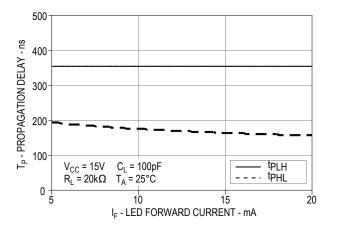
Figure 12. Propagation Delay vs. Input Current.
