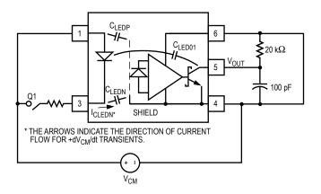
Figure 19. Not Recommended Open Collector LED Drive Circuit.
