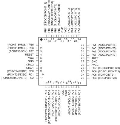
Note: The large center pad underneath the VQFN/QFN/MLF package should be soldered to ground on the board to ensure good mechanical stability.
