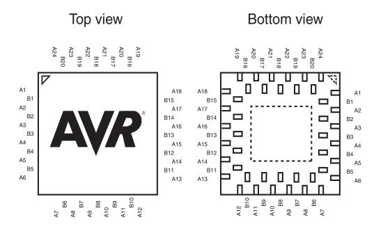
Table 1-1. DRQFN - Pinout ATmega164P/324P
