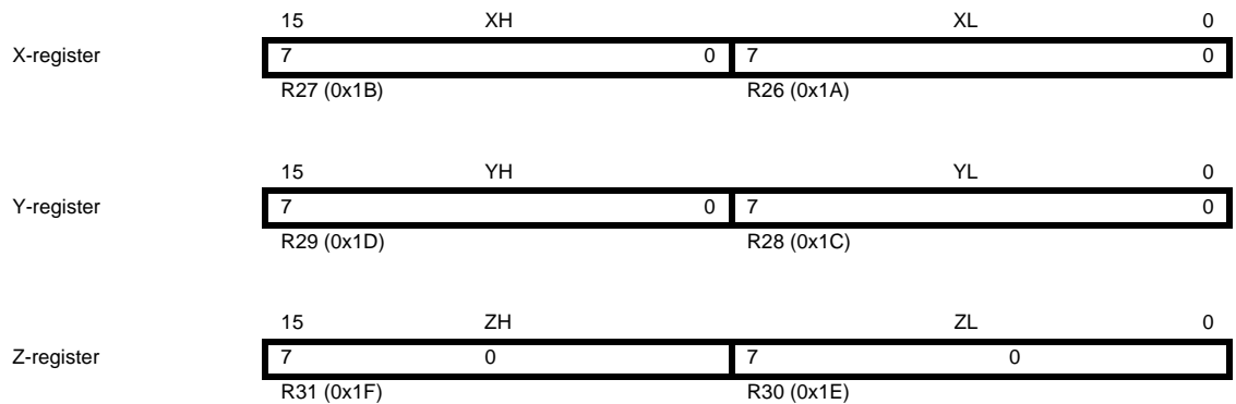
Figure 4-3. The X-, Y-, and Z-registers
