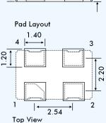
Pad Connections 1 Enable/disable 2 Ground 3 Output
