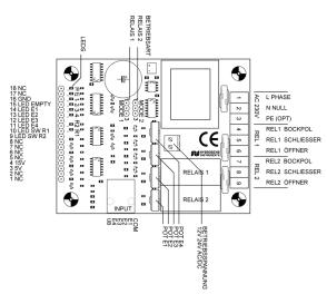
230V AC model: The connection with mains power supply should be done by only trained and authorised persons. The electrical connection is done through the 9-pin plug connector as per pin configuration. The device can be operated only with 230V AC supply. The mains supply connection is protected against over-voltage through a 390V varistor. The safety of the device against too high load current should be ensured through an external protection arrangement.
