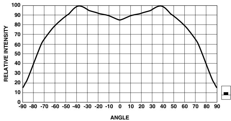
Figure 6. Relative intensity vs. angle for HSMx-C120.
