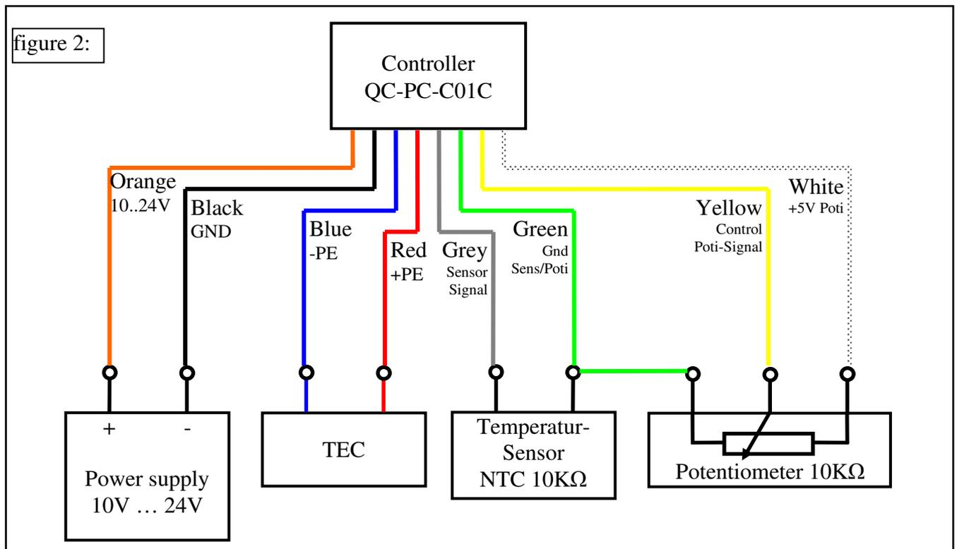
By following these instructions and using TECs from QUICK-OHM, the top side of the TEC will get cold when the right wire showing in the direction of the viewer is red. Applied on the figure above, the top side would be the warm side.
