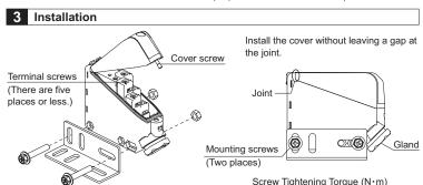
Tighten all screws surely to maintain the water-proof characteristics. (Except for UL / c-UL)
