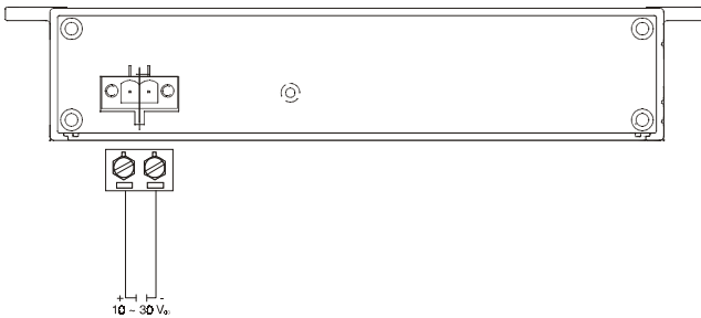
Figure 2-20 Power Connection for EDG-4504
