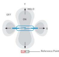
**4.3** Rotation Switch operation by **rotation** of magnet. This gives two operations per complete rotation.
