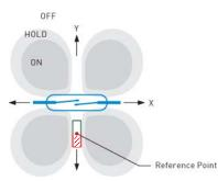
**4.2 Magnet parallel to longitudinal axis of switch.** Approaching the magnet **vertically** to the switch on the Y-axis provides one operation only. Driving the magnet over the full length of the switch (X-axis) may result in up to three operations. Minimal movement of the magnet over the switch center provides the smallest possible switching differential.
