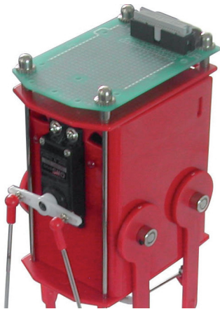
Installing experiment PCB
