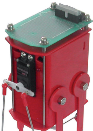
Installing experiment PCB
