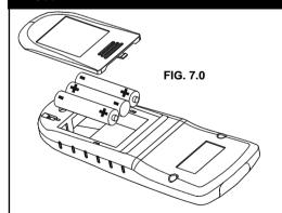
Insert the batteries in the battery compartment as indicated in fig. 8.0 and close the compartment.
