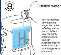
TIP: For optimal operation and longer life of the refueling station, use of distilled water is highly recommended. You can purchase distilled water from your local drugstore or pharmacy.
