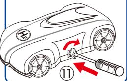
To purge the complete fuel cell power system, remove all the air out of the balloon by pulling on the syringe. Stop pulling on the syringe once all the air is removed from the balloon.
