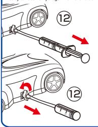
Connect the refueling station's output valve to the car's input valve turning clockwise while gently pressing in.
