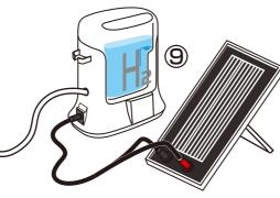
Switch the refueling station to the "A" sign. The small blue lights will now be flashing and you are now producing hydrogen fuel using unlimited power from the sun! You can see you are producing hydrogen when small oxygen bubbles form on the right side of the water tank. Turn the switch off and the hydrogen production will stop.
