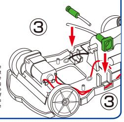
Position the fuel cell onto the square slot located in the middle of the car chassis. The positive mark on the fuel cell should be positioned on the side with the red cable, and the negative mark on the side with the black cable. Push the fuel cell into the chassis.
