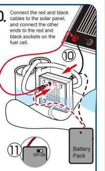
ALTERNATE OPTION: Connect the red cable from the battery pack to the red socket on the fuel cell and connect the black cable to black socket.
