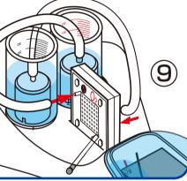
For solar panel: remove the cables connecting the solar panel to the fuel cell. Turn the switch on the battery box to "off" and remove the cables from the cable sockets located on the fuel cell. Keep the battery box switched to the "off" position except during the time you are performing electrolvsis.
