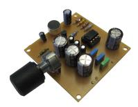
This highly sensitive microphone is able to receive after being fitted in a half-ball-shaped reflector (eg. a divided play ball) noises and words from more than some hundred meters. Ideal for observing animals, for detectives etc. Fitting case: G085 - Standard wall case
