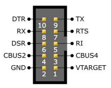
If the mainboard's connector is not being used for the USB-interface, we may connect the device to other systems – e.g. for remote controlling the robot by UART from other Microcontrollers.
