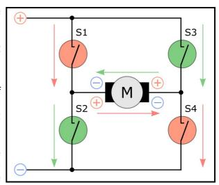
or S3 and S4 simultaneously. Each of these combinations would result in a short circuit and might destroy the activated switches.
