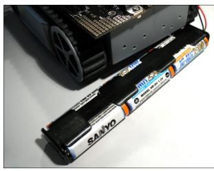
You may now insert 6 NiMH Batteries with CORRECT ORIENTATION / POLARITY!
