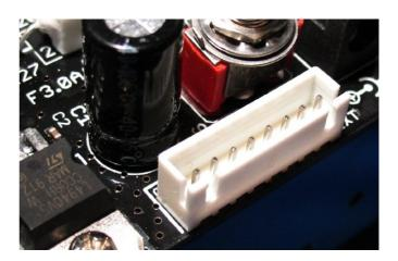
On the back of the PCB directly next to the charging connector and the main power switch is the EXT connector. It can be used to completely bridge the main power switch. This is useful for expansions like automatic charging stations or for adding more accumulators to the Robot. If you use this feature you need to turn the main power switch permanently in to position OFF.
