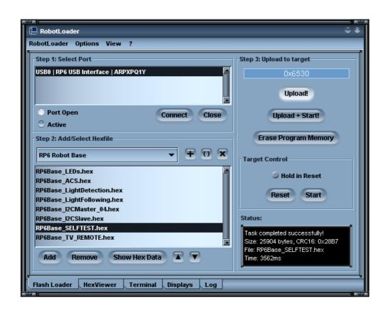
Having passed this initial check, you may now start a simple self test program in order to verify that the robot's subsystems are working properly. First you have to add the Selftest program to the Hexfile list. This can be done by pressing the "Add" Button and selecting file "RP6Base\_SELFTEST\RP6Base\_SELFTEST.hex" in the example directory. The selected file contains the self test program in a hexadecimal format – that's why such files are called "Hexfiles".
