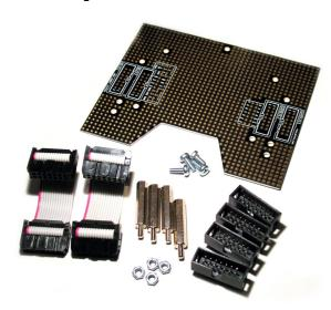
There is already an experiment expansion module for assembling your own circuits included in the delivery of the robot (only with the original RP6! Not included with RP6v2!). The module is supplied as a kit. You will have to CORRECTLY insert and solder the connectors by yourself. Pay special attention to the correct polarity - check the PCB's white silkscreen printing.
