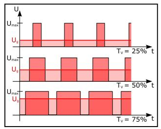
The figure shows what we can do. We generate a square wave at a *fixed* frequency and apply pulse width modulation,
