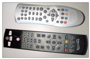
The IR receiver allows the RP6 to receive IR-signals from standard TV/Hifi remote controls, but this is restricted to remote controls using the RC5 code! Most of the universal remote controls (see fig.) may be programmed to this code – please read the manual of your remote control to set up the RC5 code. If RC5-code is missing in the code table, you may simply test several different manufacturers.
