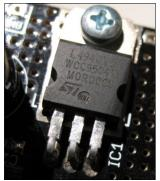
This is performed by an integrated voltage regulator capable of supplying a current up to 1.5A (see figure). At 1.5A this device would dissipate a lot of heat and therefore it is attached to a large copper plane on the PCB. Even with this heat sink we suggest to limit currents over 1A to a few seconds only. Otherwise you will have to attach an additional heat sink.
