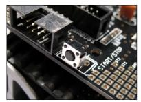
Start the program by pressing the RP6's Start/Stop Button, located near the programming connector (see fig.)! Later you can use the buttons in RobotLoader Software or use the keyboard shortcut [STRG]+[S], but by using the hardware button now, you can directly verify that it works OK.
