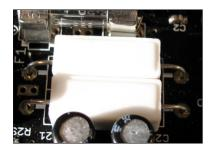
Each of the two motor current sensor circuits contains a power resistor. Ohm's Law  $U=R\cdot I$  tells us that the voltage drop at a resistor is proportional to the current flow through it!
