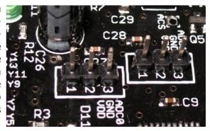
**ATTENTION: The Pinout is NOT compatible with standard Servos!** This is on purpose as you need some power supply filtering for most Serovs anyway (LC Lowpass Filter for example – so for example 10 to  $100\mu H$  ferrite core high power inductor / choke in series and  $220\mu F$  capacitor parallel after the inductor close to the servo).
