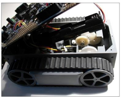
You do NOT need to unplug the tiny 3-pin connector of the bumper PCB (see fig.)! Be careful to touch the main board at the edges and at larger plastic parts only in order to avoid static discharges!
