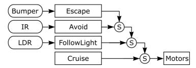
The priority or "FollowLight" is below Escape and Avoid, but above Cruise, which implies the "Cruise" behaviour will never be activated in this example unless the room is very dark (as soon as both LDR-levels drop below 100, the "FollowLight" behaviour will be deactivated).
