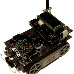
On the two images on this page you can see the RP6 with two expansion modules (Experiment PCB and RP6-M32 with LCD) and the new RP6v2 with RP6v2-M256-WIFI (of course it can also be used on the old RP6!), Antenna and LCD. The new connectors are shown in more detail in the appendix.
