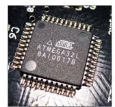
As you can see in the diagram, the robot's central unit is an ATMEL ATMEGA32 8-Bit Microcontroller (see fig.).
