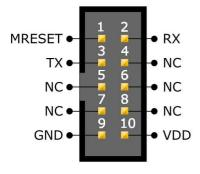
Of course RX and TX must be interchanged to allow communication. Additionally, the connector orientations had to be mirrored to allow a correct orientation for the protecting pull-relief of the flat ribboncable's plug.
