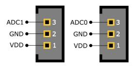
We did not assemble these connectors and you may apply use 3-pin connectors with 2.54mm grid. Be careful in soldering and do not ruin the mainboard! If you are unexperienced with soldering, please refrain from soldering at the mainboard and prefer to start experiments by using an expansion board!
