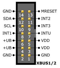
The figure shows the connection diagram for both expansion connectors. On the mainboard, pin 1 is always located near the white label XBUS1 and XBUS2, respectively. Alternatively, the pin is labelled with "1" at the connector-position.
