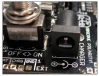
You can see a polarity marking on the mainboard in front of the plug (see figure). The negative terminal is located on the OUTER METAL PLATE and the positive terminal on the INNER pin!
