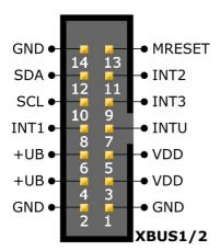
For the sake of completeness we start by defining the connector pin assignments for the expansion connector once again (s. chapter 2):
