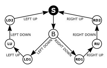
The state machine starts at state S and immediately transits to state B (while displaying a short text message). Having arrived at state B the system will wait until you hit one of the bumpers.
