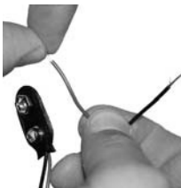
Figure 26: First twist the strands between your fingers.
