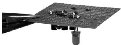
Figure 63: Cut off the connection wires closely to the solder cones.
