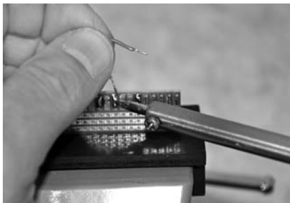
Figure 35: Pull slightly on the wire with your fingers while heating the soldering area, until the wire comes loose.
