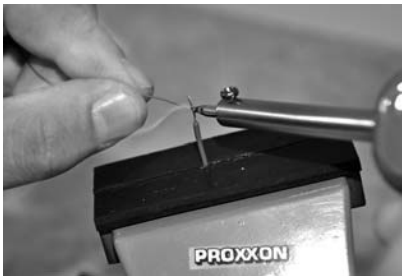
Figure 27: The twisted wire must be heated and some solder added, which melts at once.
