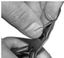
Figure 29: The wire bent to shape with an electrician's round pliers.
