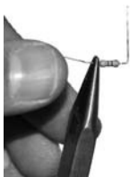
Figure 30: For electrical components, the wires should not be bent right at the casing end.
