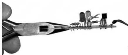
Figure 62: The cut connections should protrude over the PCB by 0.5 to 1 mm.
