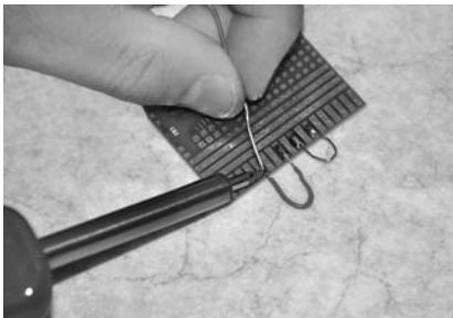
Figure 31: Soldering wire bridges to the lateral strip grid
