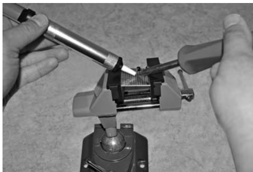
Figure 65: De-soldering requires the de-soldering pump.
