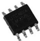
Figure 16: At the SMD-IC, PIN 1 is marked by a point at the top of the casing.
