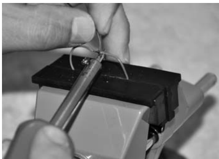
Figure 28: Since the insulation melts quickly, the wires must be soldered together quickly.
