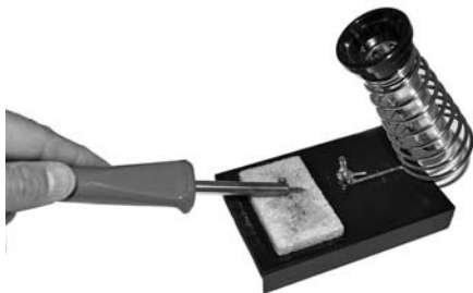
Figure 25: Therefore, contaminations need to be wiped off regularly with the moist sponge.
