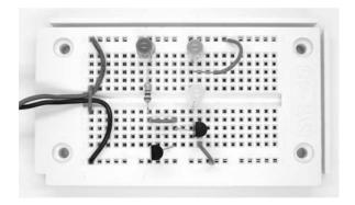
Fig. 27: Transistor as temperature sensor (Aufbau8.jpg)
