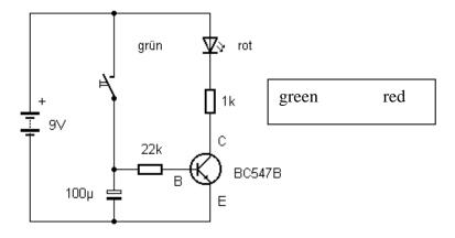
Fig. 16: Delayed switching-off (Schaltung3.jpg)
