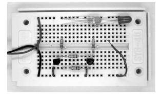
Fig. 29: The flip-flop (F\_Flipflop1.jpg)
