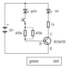
Fig. 12: An NPN transistor in the emitter circuit (Schaltung1.jpg)
