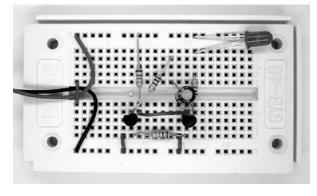
Fig. 35: The LED flasher (F\_Blinker2.jpg)
