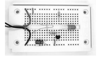
Fig. 17: The afterglow electric torch (F\_NPN3.jpg)
