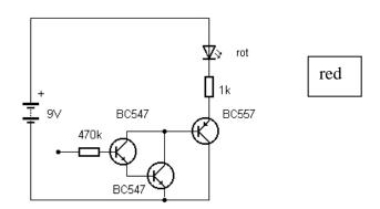
Fig. 20: Current gain with three transistors (Schaltung5.jpg)
