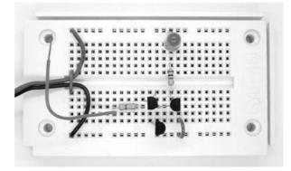
Fig. 21: Sensor amplifier for electric fields (Aufbau5.jpg)
