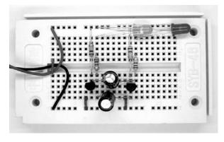
Fig. 33: A slow alternating flasher (F\_Blinker1.jpg)
