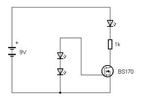
Fig. 44: LEDs as photovoltaic cells (Schaltung17.jpg)
