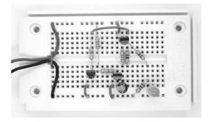
Fig. 37: LED flashing light (Aufbau13.jpg)
