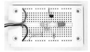
Fig. 15: Examining the current gain of the BC557 (Aufbau2.jpg)
