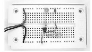
Fig. 47: The temperature sensor (Aufbau18.jpg)
