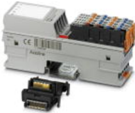
Axioline digital output terminal, 8 outputs, 24 V DC, 2 A, 2-wire connection method (including bus base module and plugs)
