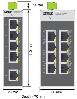
Figure 5 Housing dimensions
