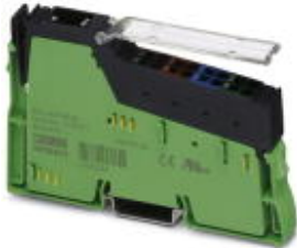
Inline power terminal block, complete with accessories (plug and labeling field), 24 V DC, with fuse (Main and segment voltage) and diagnostics
