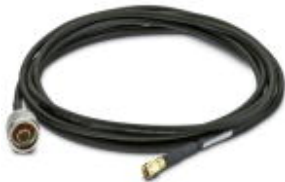
Antenna cable, 0.5 m in length; N (male) -> RSMA (male), impedance 50 ohms
