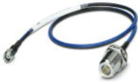
Adapter cable, pigtail 50 cm, N (female) -> RSMA (male), insertion loss 0.75 dB at 2.4 GHz; 1.25 dB at 5 GHz, impedance 50 Ohm;
