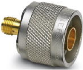
Adapter, N (male) -> SMA (female); insertion attenuation < 0.3 dB at 2.4 GHz
