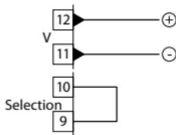
Linear output in Volt configurable using parameters as command (Parameter *c.out*) or retransmission of process or setpoint (Parameter *rEtr*).
