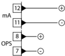
Pins 11-12: linear output in mA configurable using parameters as command (Parameter *c.out*) or retransmission of process or setpoint (Parameter *rEtr*).
