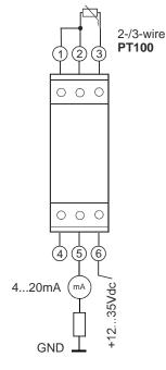
The output current follows linear at the input
