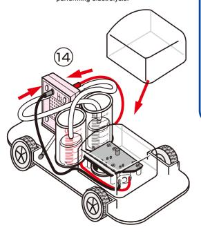
Connect the red and black cables to the solar panel, and connect the other ends to the red and black sockets on the fuel cell.
