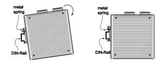
To remove the device from the DIN-Rail, simply reverse Steps 1 and 2 above.
